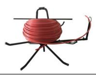
7.Pull out the spring sleeve at the bottom of the center of the swivel frame and insert the two pressure rods into the sleeve to hold down the coil.
